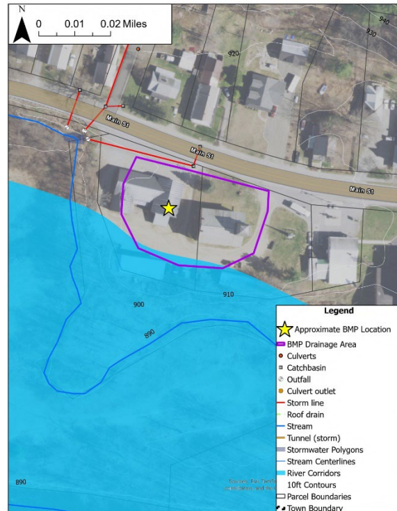
Figure 13. The drainage area for the Cavendish Historical Society Museum site is shown outlined in purple. The location for the proposed bioretention practice is depicted with a yellow star.
